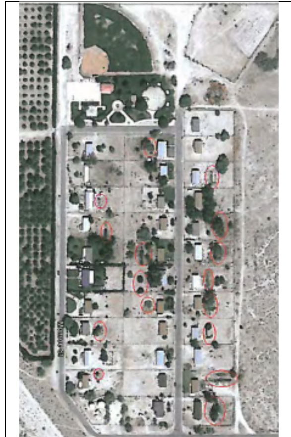
Failing Septic Systems (Circled in Red) at Ave 64 Housing
